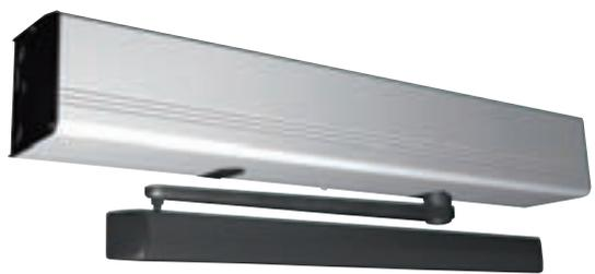
**ABLOY® EMSW** swing door operator works electro-hydraulically. It opens by motor and closes by spring. It is suited for external, internal, fire and exit doors, also for large and heavy doors.
